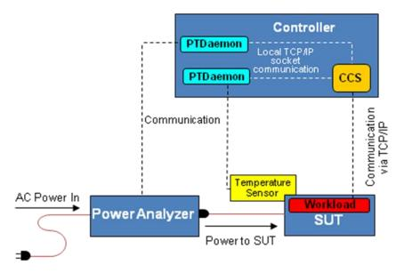
As options beyond this picture, the JVM director could run on any of these systems or even another one, with appropriate configuration and property file changes. The PTDaemon components controlling the power analyzer and temperature sensor could run on the SUT or even a separate system from the benchmark controller system.
